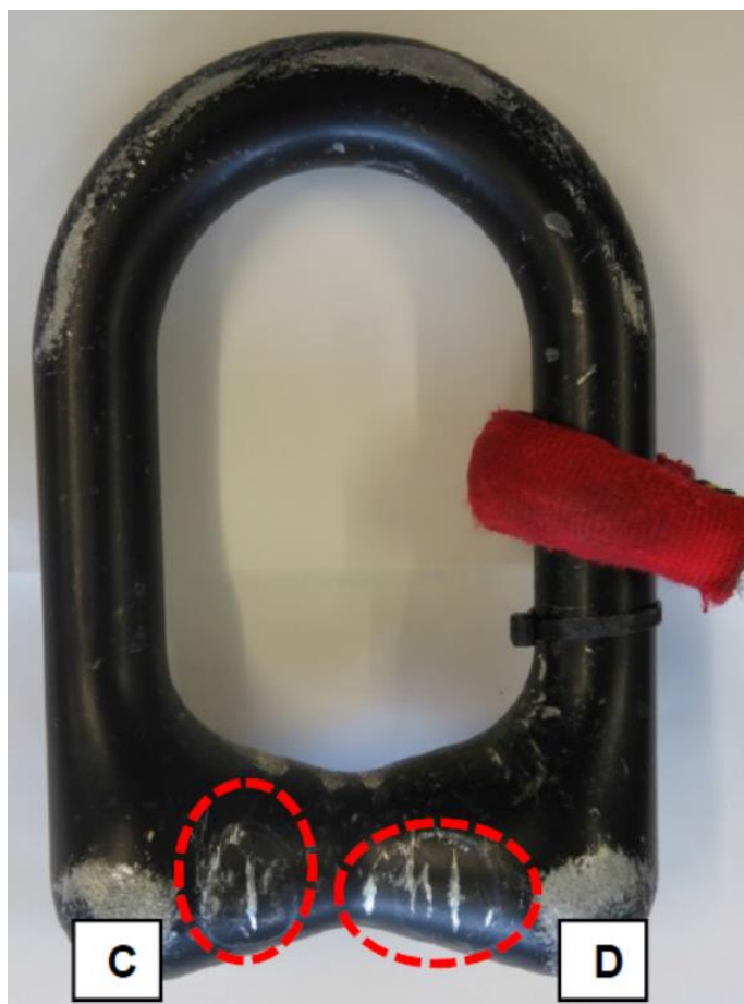
Fig.15 – Main hook ring - Example significate damages
