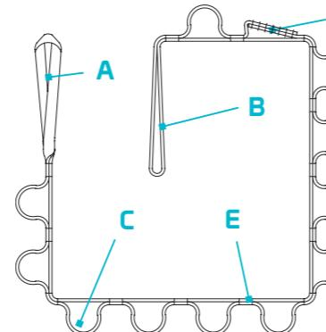
**EN:** (A) Lark's foot loop, (B) End loop, (C) Adjustment loop, (D) Main stitch, (E) Secondary stitch.
